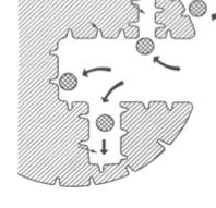
The core of the technology is the use of a weakly acidic matrix platform with medium to large pore, ultrastable small grain molecular sieve, a micro-mesomacro pore structure by anti-metallic components, and catalytic cracking catalyst with an adjustable active site. It enables efficient conversion of heavy oil with lower coke in the reaction process to reduce carbon emissions during catalyst regeneration.
